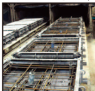
□ 석재판 부착과정 Stone plate attachment process
